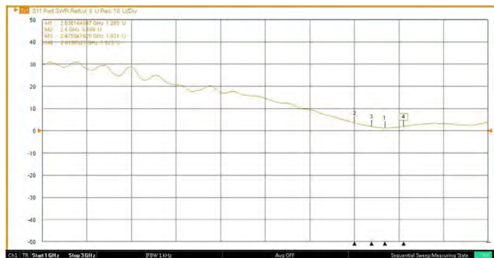
Fig. 11. VSWR measurement results for double E-shaped microstrip antenna
