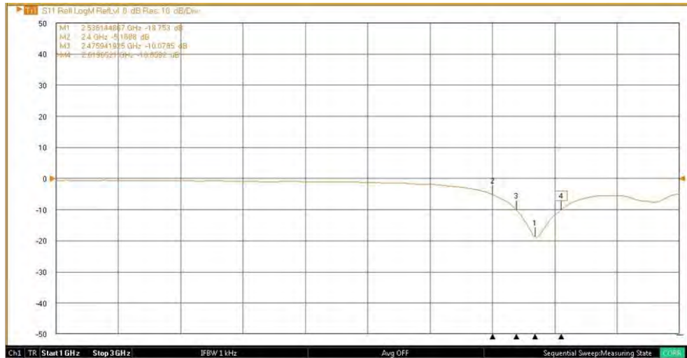
Fig. 10. The results of the return loss measurement of the double E-shaped microstrip antenna
