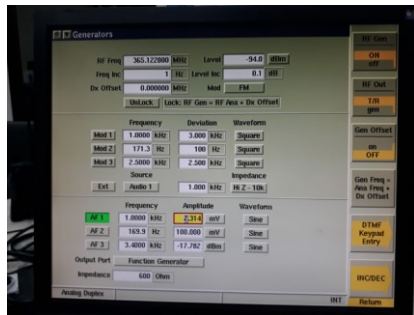
Fig. 10. The display of the settings on the Audio Frequency Generator
