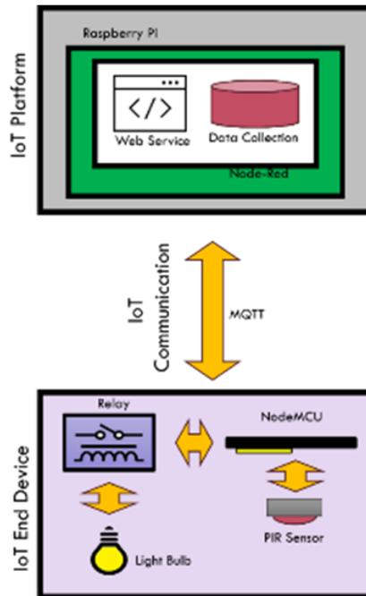
Figure 2: The IoT-based smart lighting control block diagram.
