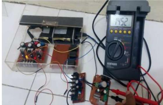
Figure 13: Measurement DC-DC step down converter.
