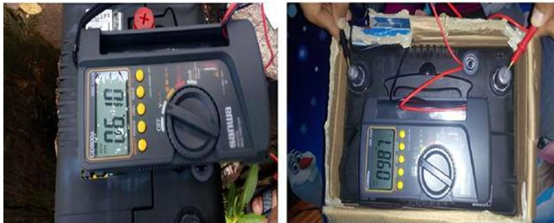
Figure 12: Results of testing battery condition (a) bad and (b) good enough.
