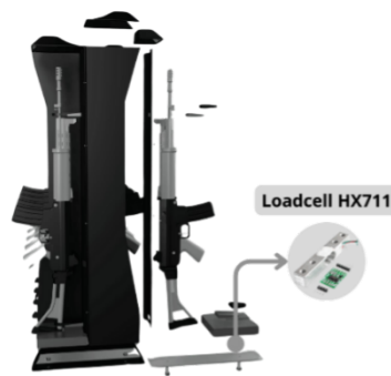
Figure 2: Load cell sensor position.
