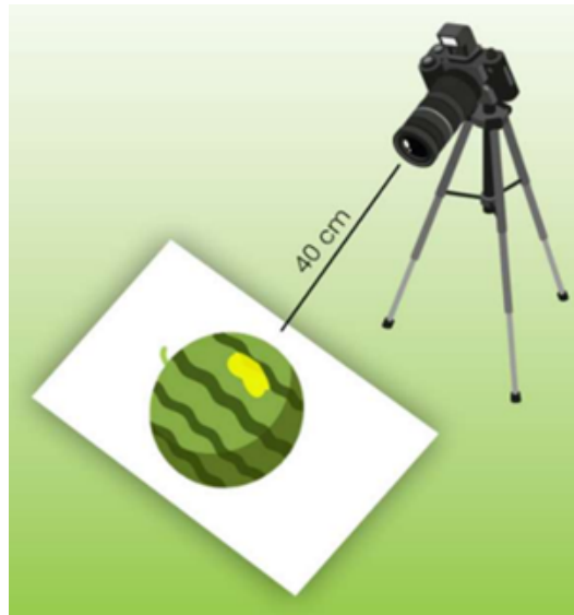
Figure 4: Data acquisition setup for the watermelon dataset.
