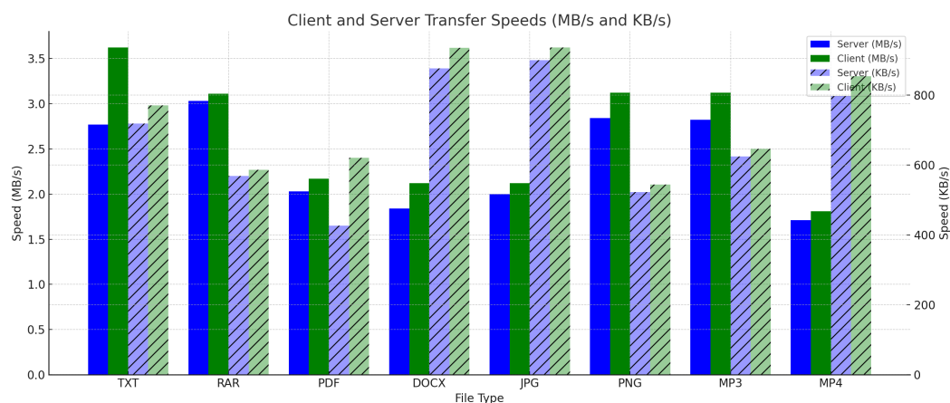
Figure 6: Comparison of transfer speed between client and server in the same (KB/s) and different (MB/s) file size group.
