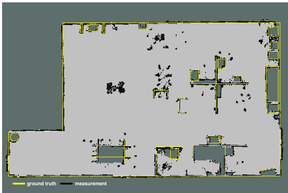
Fig.10. 2-D Mapping Results by The Mobile Robot Using 2-D LIDAR Sensor Based on HECTOR SLAM Method on The ROS Platform.
