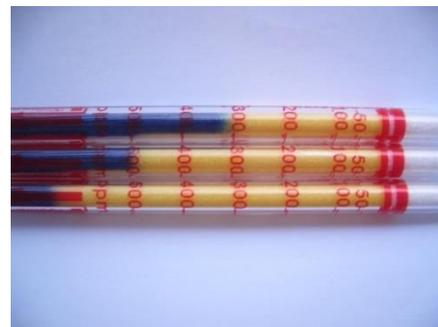
Fig.11. Ozone Output Measured by the Colorimetric Method.
