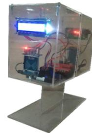
Fig.4. RFID System Device.
