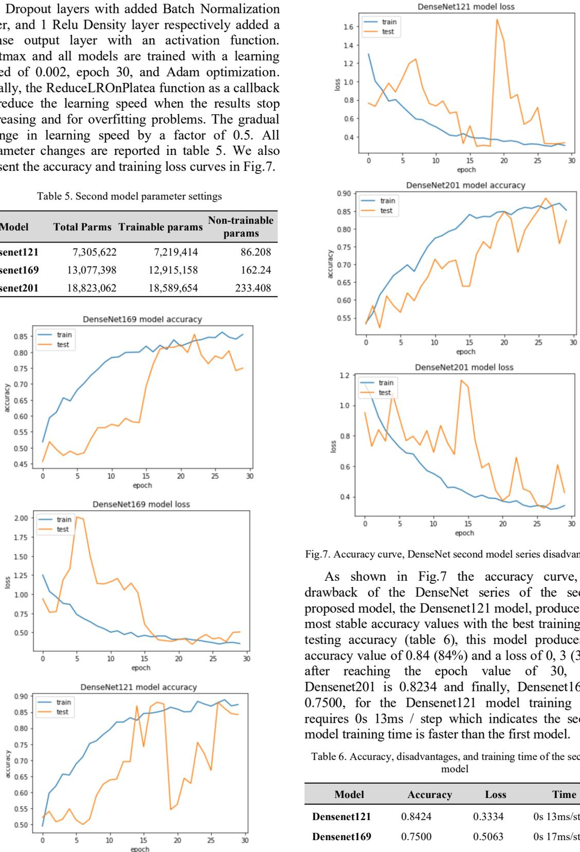
Fig.7. Accuracy curve, DenseNet second model series disadvantages
