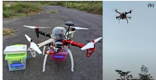
Fig. 7. Unedited photos for drones (a) before take-off and (b) successfully hovered and collected data
