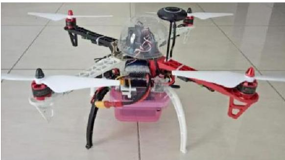
Fig. 6. Assembled drone with an F450 frame and equipped with Arduino meteorological sensors as a payload
