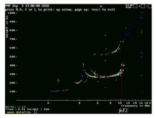
Fig.1. Example of an ionogram observed using CADI ionosonde at Pameungpeuk station, September 3, 208, at 13.00 WIB
