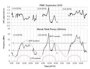
Fig.7. The graph of *foF2* depression (r) above Pameungpeuk from September 1 to 3, 2019 (top panel) and the correction results for MUF predicted using ASAPS software, for the Merak - Teluk Penyu communication circuit.
