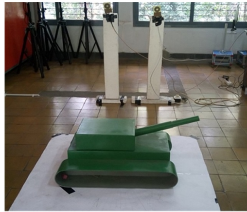
Fig. 6. Experimental measurement of antenna and tank miniature configuration.
