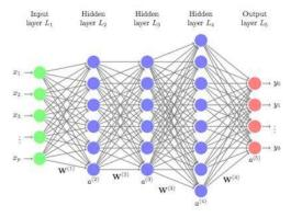
Fig. 6. The architecture of multi-layer perceptron.
