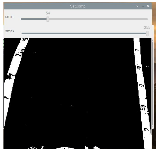
Fig. 11. Saturation threshold test.
