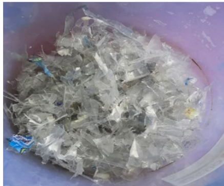
Fig. 5. The result of shredded PET type plastic which is chopped using a shredder machine.
