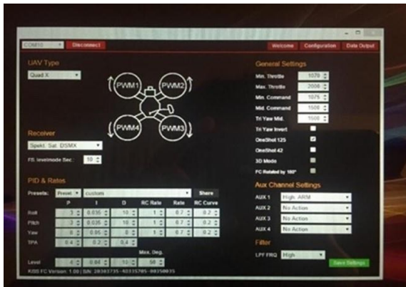
Fig. 1. Application to determine the PID value on the controller.
