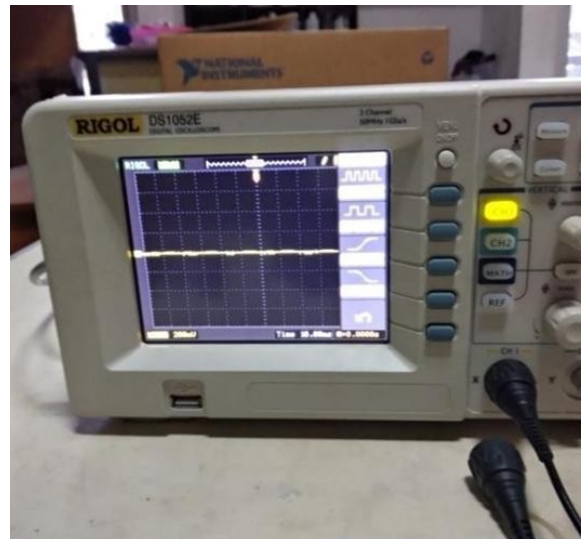
Fig. 6. Testing motor response using an oscilloscope during motor standby conditions (1 Volt).
