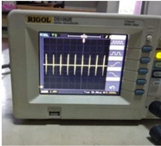
Fig. 7. Testing motor response using an oscilloscope during motor standby conditions (2 Volts).
