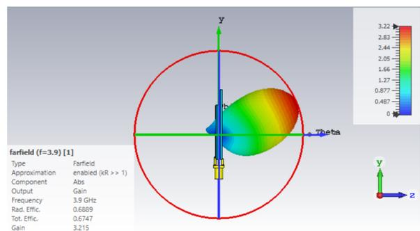
Fig. 7. Radiation pattern of proposed resonator.
