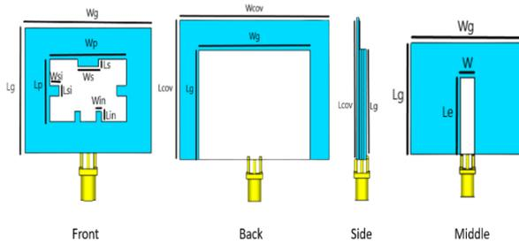
Fig. 2. Wearable resonator design in CST.
