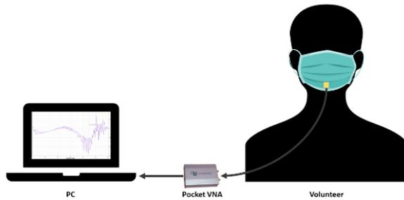
Fig. 4. Prototype of measurement setup.
