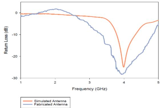
Fig. 5. Comparison of simulated and measured resonator.
