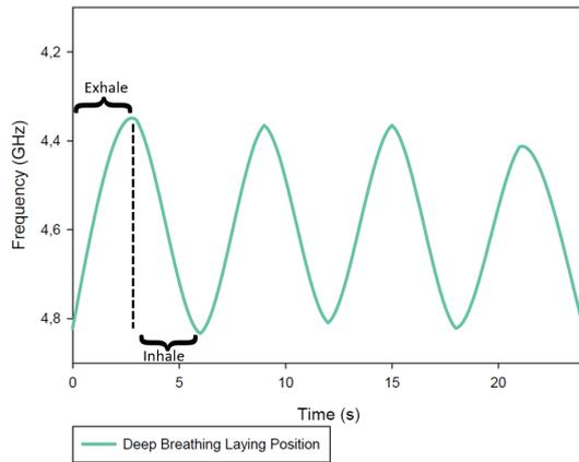
Fig. 8. Measurement of deep breathing in laying down position.
