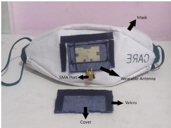
Fig. 3. Wearable textile jeans-based resonator mask.
